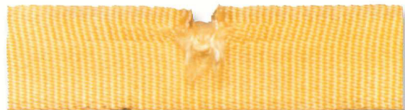
Damage caused by sharp edges on sides
