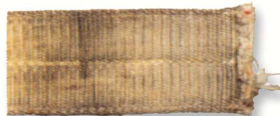
Damage caused by sharp edges
