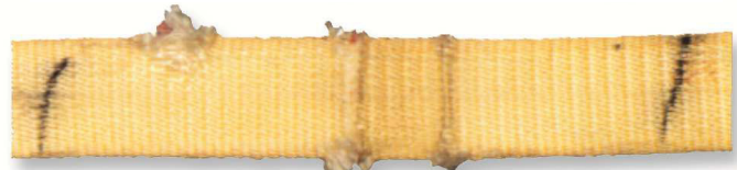
Damage caused by sharp edges in one face
