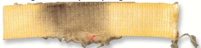
Damage caused by burning
